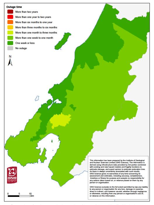
Figure 6.10 Outage times for telecommunication services (data, cellular and landline) in the base-case.
