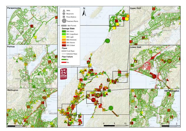
Figure 6.14 Modelled damage to the Wellington Region water network.
