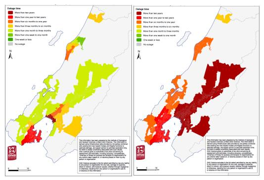
Figure 6.20 Outage times for waste water collection (left) and treatment (right) for low and high investment programmes.
