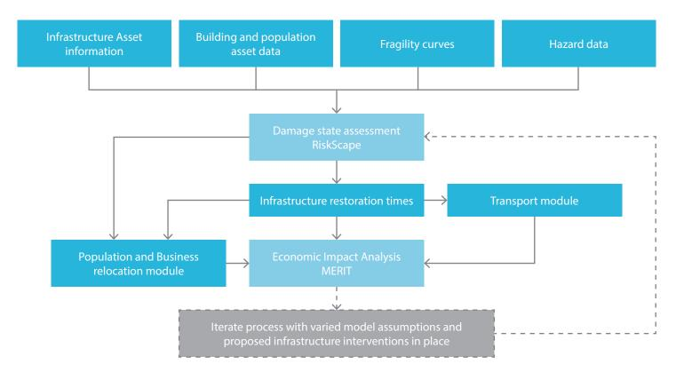
Figure 9: Linkages between the various stages of damage loss assessment and economic impact analysis
