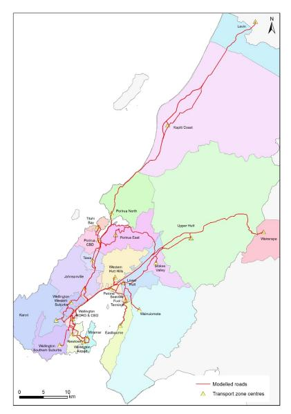
Figure 5.1 Transportation zones and routes selected for damage modelling.
