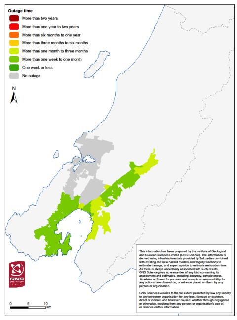
Figure 6.23 Outage times for gas to critical and general customers.
