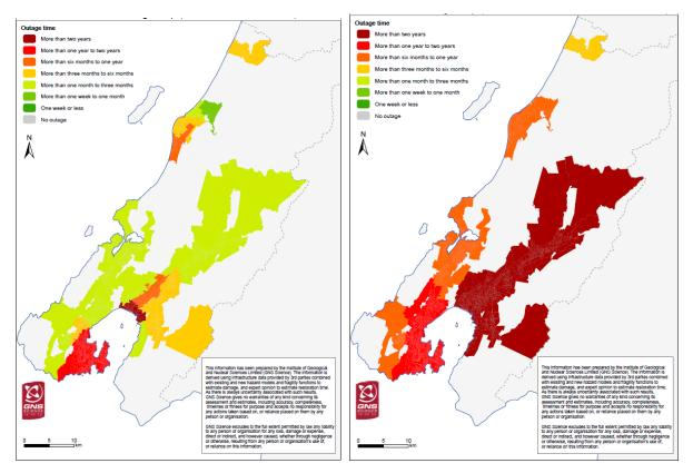
Figure 6.21 Outage map for waste water collection (left) and treatment (right) for the preferred programme.
