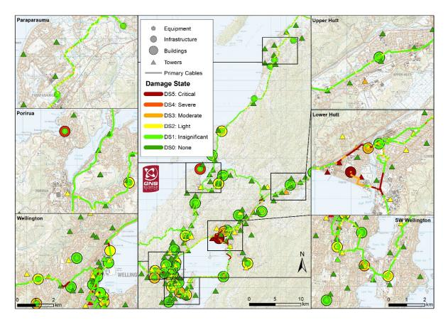
Figure 6.9 Modelled damage to the Wellington Region telecommunications network.
