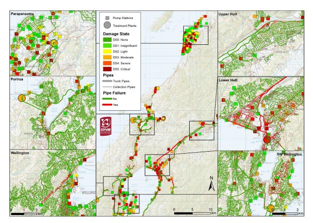
Figure 6.18 Modelled damage to the Wellington Region waste water network.
