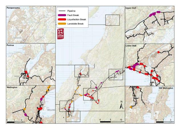
Figure 6.22 Modelled damage to the Wellington Region gas network.
