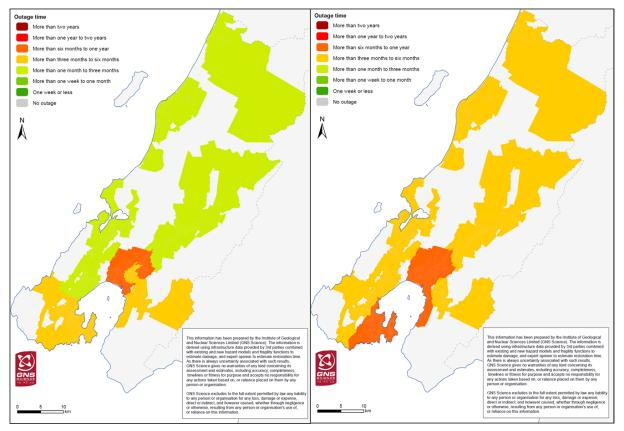
Figure 6.15 Outage map for non-potable (left) and potable (right) water services.
