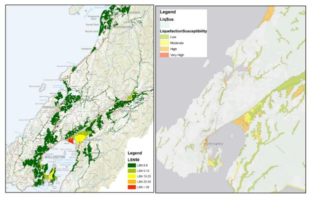
**Figure 4.3** Mean LSN (left) and liquefaction susceptibility (right) values for the Wellington Fault scenario (Dellow, Perrin and Ries, 2015).
