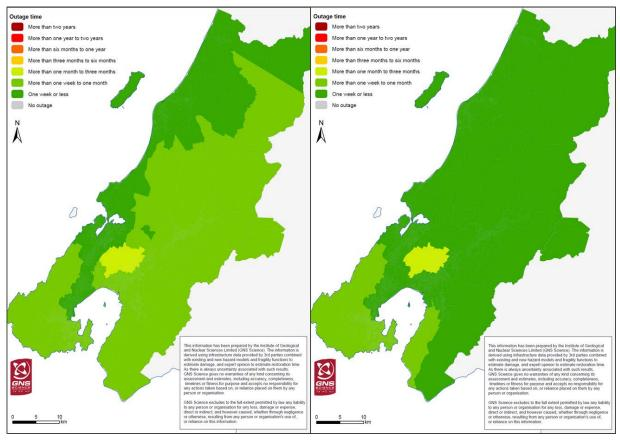
**Figure 6.11** Outage times for telecommunication services (data, cellular and landline) for low (left) and high (right) investment programmes.
