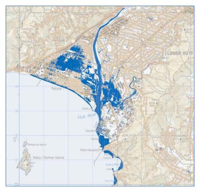
**Figure 4.6** Estimated subsidence (dark blue) extent (areas below MSL) resulting from a M7.5 Wellington Fault earthquake (based on Townsend *et al.*, 2016).
