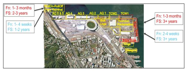
**Figure 5.5** Restoration times for port assets in Wellington. Red text is base-case outage times, blue text is intervention and preferred programme outages.
