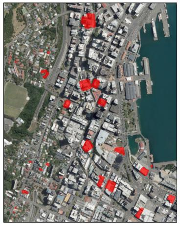
**Figure 7.2** Example of cordon zones (red) in Wellington CBD associated with > DS4 buildings for a single scenario realisation.
